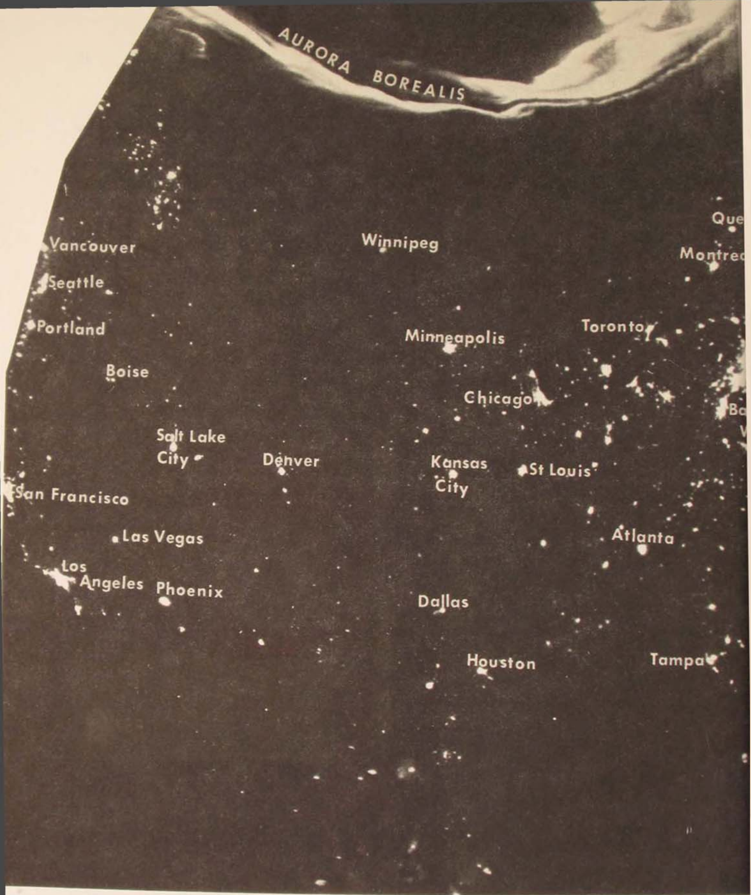
Figure 1. A nighttime montage of North America depicts city lights and the aurora borealis, from a DAPP high-resolution sensor on two revolutions of a synchronous satellite. Besides enabling new research on the aurora and its effects, information can be gleaned from such imagery for use in geographical gridding, forest fire detection, light pollution, energy evaluation, electrical storm detection, volcanic location, oil field intelligence, and many other areas of investigation.
